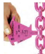
Checking pitch extension due to nominal thickness wear
