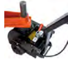
Mechanical travel positioner for travel support and exact positioning
