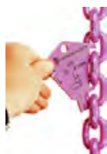
Checking plastic extension due to overload
