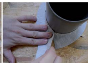
Overlap the end of the adh. tape with the front of the adh. tape
