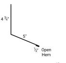
Profile Code: NS Detail Code: 07 Detail Num: EW Girth Num: 10.25" Provide Roof Pitch
