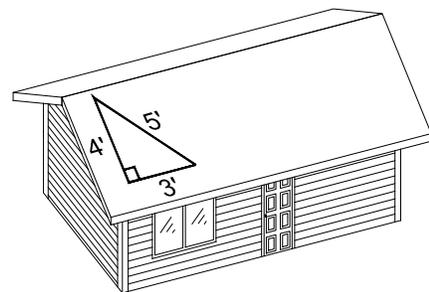
*It is important to measure the roof from gable to gable. Proper placement of panels will allow the panel ribs on each side to be covered by the gable trim while creating a symmetrical appearance on the roof.*
