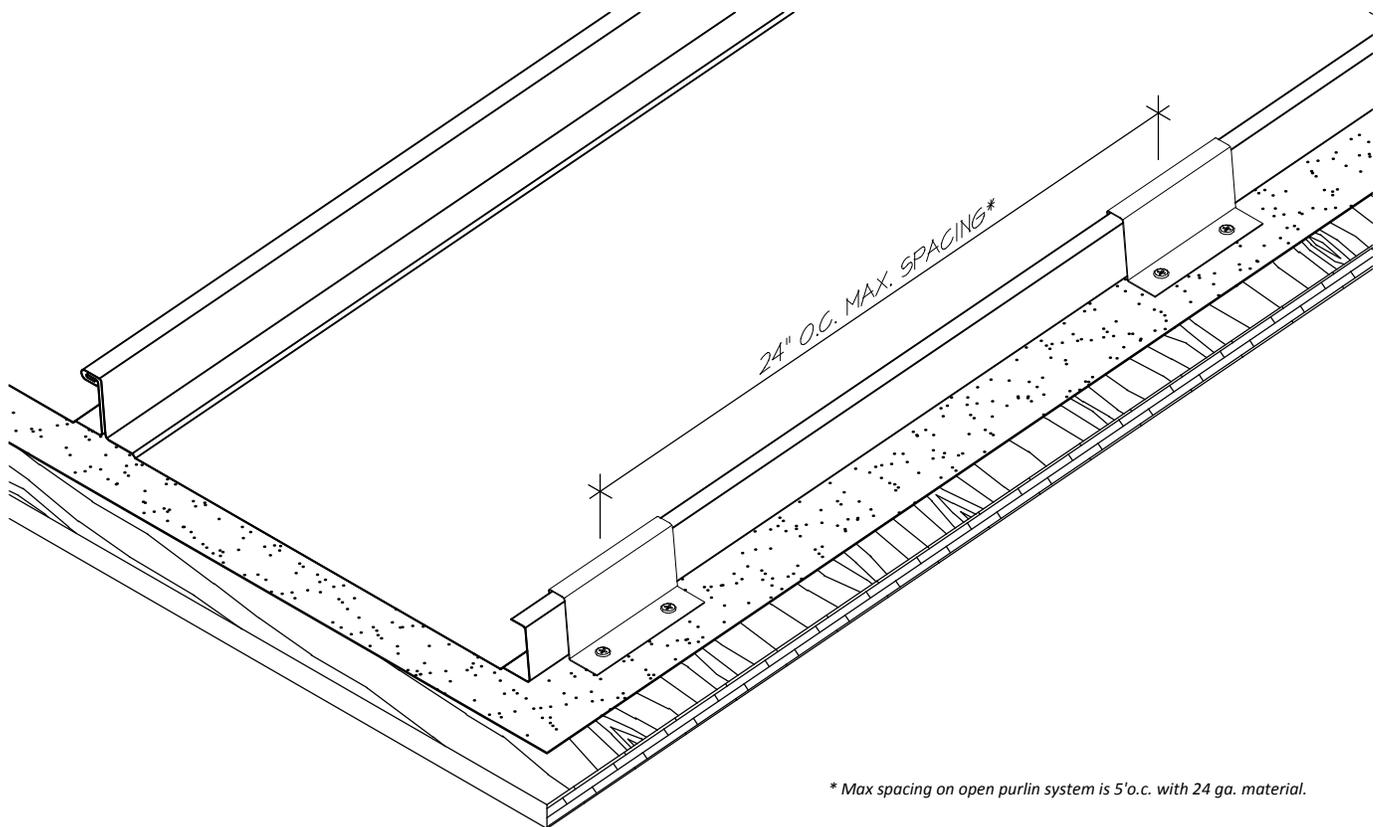
*\* Max spacing on open purlin system is 5'o.c. with 24 ga. material.*
