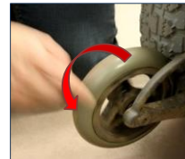
Spinning the anti-tip caster
