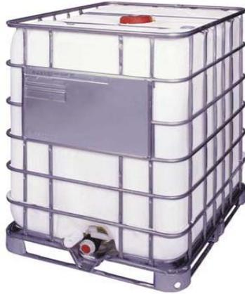
Our Polyethylene Composite IBCs are composed of an inner container extrusion blow-molded from high density polyethylene and an outer container made of rigid welded galvanized tubular steel grid. They work well with steel, wood or plastic pallets.
