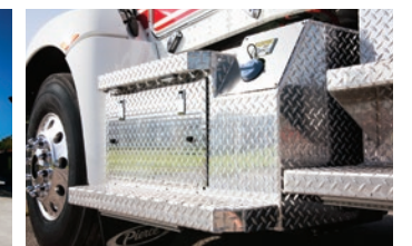
Rear fuel tank – batteries in step
