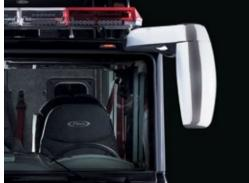
With no center post obstruction, the single-piece windshield opens sight lines and reduces risk of accidents with clear views of the road, pedestrians, and traffic. Available on Enforcer<sup>™</sup>, Impel<sup>®</sup>, Saber<sup>®</sup>, and Velocity<sup>®</sup> custom chassis.
