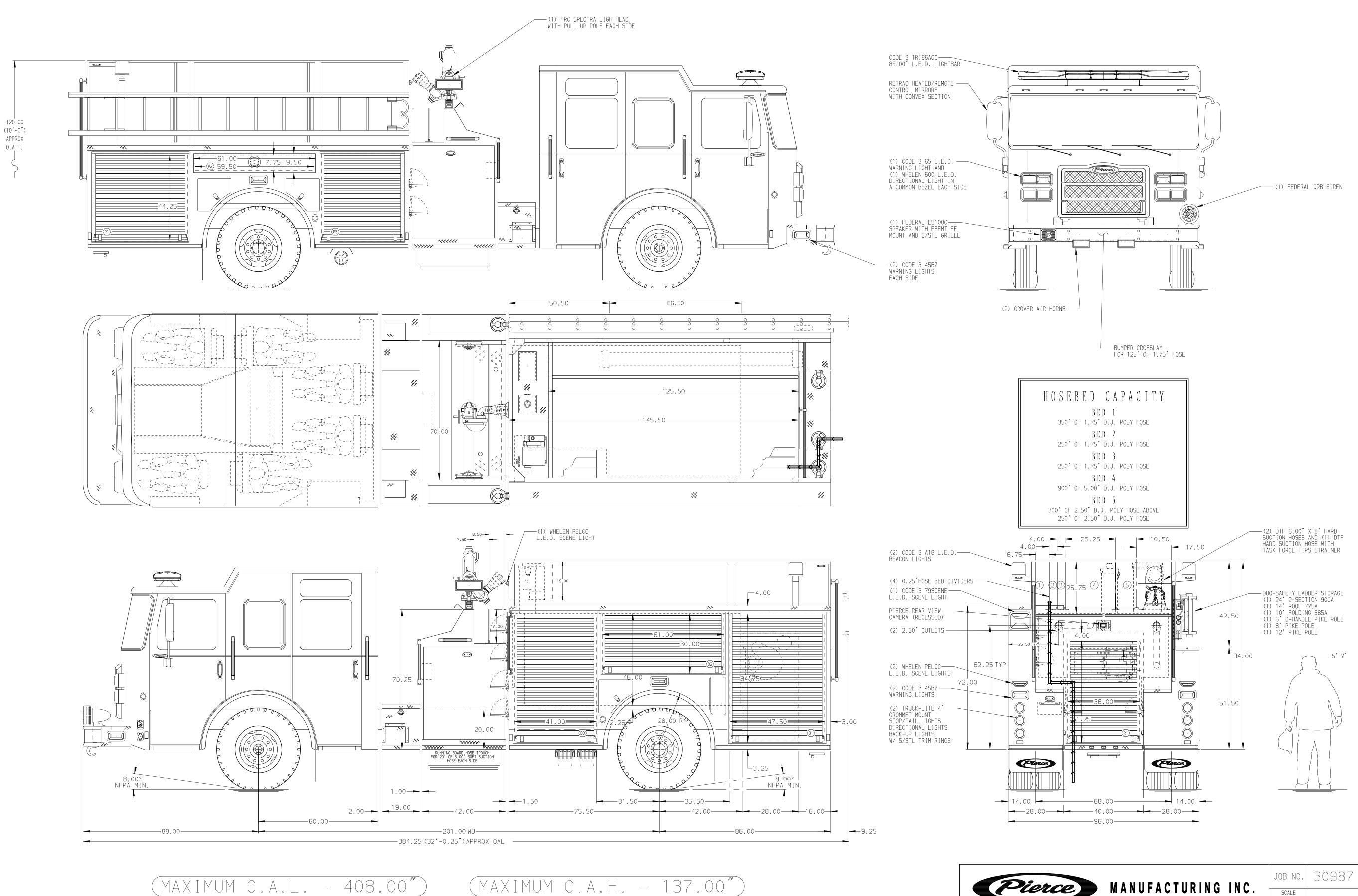
DIMENSIONS SHOWN ARE APPROXIMATE AND ARE SUBJECT TO MINOR DEVIATIONS 1. ONE 1.50 OUTLET WITH 2.00 PIPING AND SWIVEL LOCATED IN BUMPER CROSSLAY HUSKY 3 RESERVOIR LOCATED PER SHOP ORDER SHORELINE RECEPTACLE WITH KUSSMAUL SUPER AUTO-EJECT LOCATED ON DRIVER SIDE CAB CORNER
