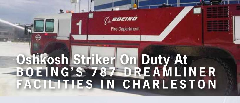
An Oshkosh Striker 6 x 6 aircraft rescue and fire fighting (ARFF) vehicle has been delivered to provide emergency response and fire protection services for The Boeing Company at its expanded Charleston, South Carolina facility that is dedicated to the 787 Dreamliner aircraft. The Striker will serve on standby for engine runs, fueling, taxiing and anywhere an emergency may occur.
