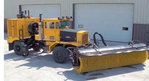
The **Fort Dodge Regional Airport** takes delivery of an Oshkosh® MPT-Series™ truck. This unit features a 315 HP Cummins® ISC 8.3L engine, Allison® RDS 3066 Automatic Transmission, 20,000 lb Oshkosh® front axle, and 23,000 lb rear axle. As well as an 18' Oshkosh Snowplow, Oshkosh Universal Hitch and 16' Power Broom and Air Blast System. For more information contact: Tom Carle [tcarle@oshruck.com](mailto:tcarle@oshruck.com).
