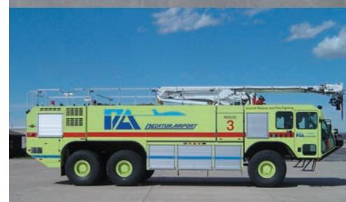
The **Decatur Airport** recently took delivery of a Striker® 3000 ARFF vehicle. The apparatus features a SNOZZLE® extendable turret, forward looking infrared (FLIR) camera and 450 lb. "Purple K" chemical agent system. The vehicle also features TAK-4® independent suspension, a 3,000 gallon water tank and a full 17 inches of ground clearance. For more information contact: Tom Carle [tcarle@oshruck.com](mailto:tcarle@oshruck.com).
