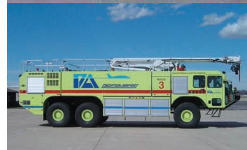
The **Decatur Airport** recently took delivery of a Striker® 3000 ARFF vehicle. The apparatus features a SNOZZLE® extendable turret, forward looking infrared (FLIR) camera and 450 lb. "Purple K" chemical agent system. The vehicle also features TAK-4® independent suspension, a 3,000 gallon water tank and a full 17 inches of ground clearance. For more information contact: Tom Carle [tcarle@oshtruck.com](mailto:tcarle@oshtruck.com).
