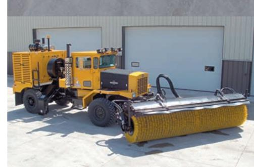
The **Fort Dodge Regional Airport** takes delivery of an Oshkosh® MPT-Series™ truck. This unit features a 315 HP Cummins® ISC 8.3L engine, Allison® RDS 3066 Automatic Transmission, 20,000 lb Oshkosh® front axle, and 23,000 lb rear axle. As well as an 18' Oshkosh Snowplow, Oshkosh Universal Hitch and 16' Power Broom and Air Blast System. For more information contact: Tom Carle [tcarle@oshtruck.com](mailto:tcarle@oshtruck.com).
