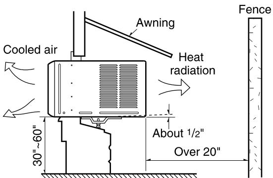
**CAUTION:** DO NOT cover or block any of the side louvers. All side louvers of the cabinet must remain exposed and unobstructed to the outside of the structure.
