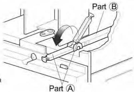
**NOTE :** Before using the ventilation feature, position the lever, as shown. First, pull down part (A) to horizontal line with part (B)
