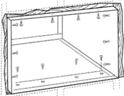
**C** Place the case in the wall opening and place wood support strips between the case bottom and the flashing on both sides of the bottom rail. They should be the same height as the bottom rail and the same length as the wall opening.
