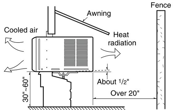
**CAUTION:** DO NOT cover or block any of the side louvers. All side louvers of the cabinet must remain exposed and unobstructed to the outside of the structure.
