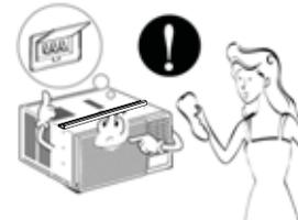
**Do not operate the unit without the air filter or when the front intake grille has been removed.**
