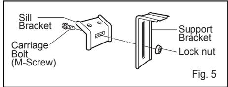
2. Attach the sill bracket to the window sill using the screws (Type B).
