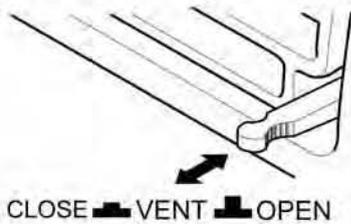
**NOTE :** Before using the ventilation feature, position the lever, as shown. First, pull down part (A) to horizontal line with part (B)
