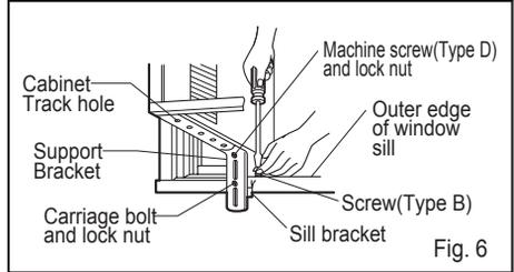
3. Using the M-screw and the lock nut, attach the support bracket to the cabinet track hole. Use the first track hole after the sill bracket on the outer edge of the window sill. Tighten the carriage bolt and the lock nut. Be sure the cabinet slants outward.
