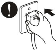
**Do not operate or stop the unit by inserting or pulling out the power plug.**
