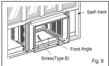
3. Pull each Frame curtain fully to each window sash track, and pull the bottom window sash down behind the Top retainer bar until it meets.
