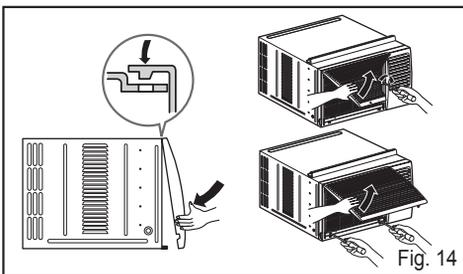
9. Lift the inlet grille and secure it with a screw (Type A) through the front grille. (See Fig. 14)
