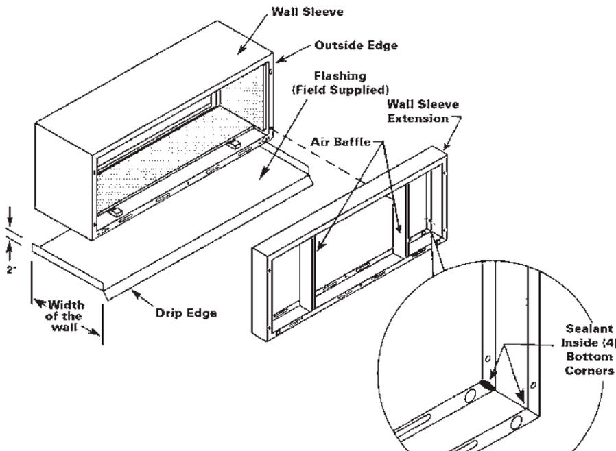
Seal condensate drip pan to wall sleeve with sealant on all (4) bottom corners.
