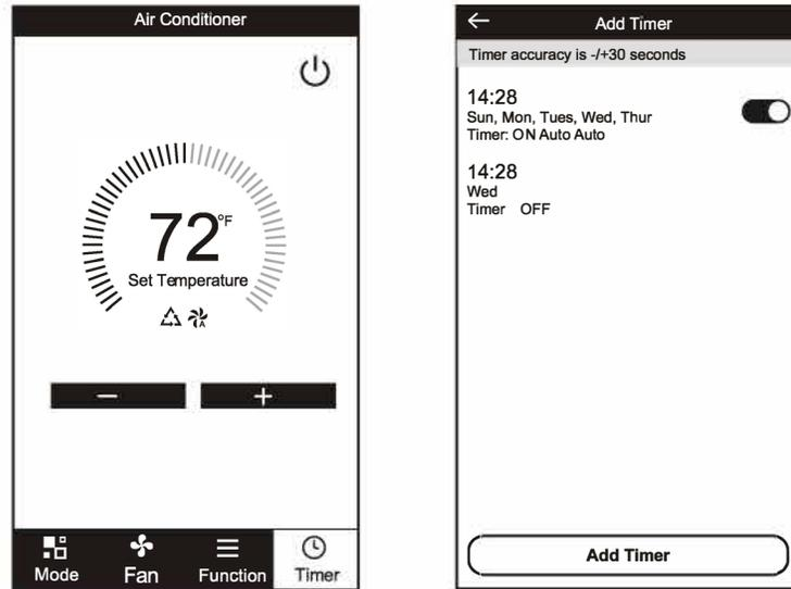
6. Click "ON" or "OFF" button to set Timer ON or Timer OFF. You can set the: Hour, Minute, Operate Mode, Operate Fan Speed, Operate Temperature. You can also set a weekly timer. After you're finished setting the timer, click the button to Cancel or Confirm
