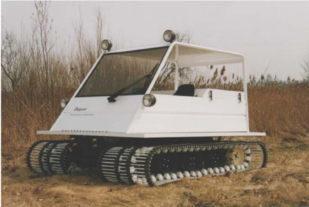
Example of the rubber block chain used as travelling gear.
