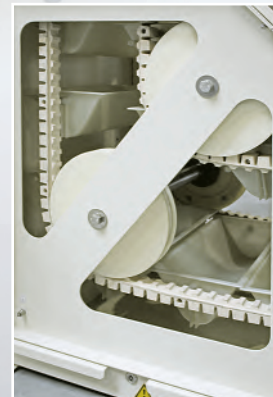
Transition from horizontal to vertical conveying
