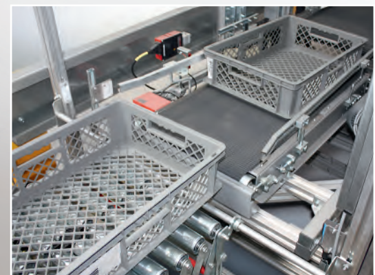
Feed station of a portal lifter with transfer onto the pivoting infeed conveyor which also singulates the items.
