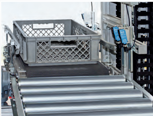
Transfer from the belt conveyor on the hoist carriage to the take-away roller conveyor
