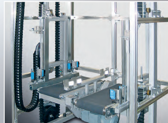
Twin belt conveyors can be supplied as an option for higher throughputs
