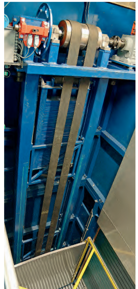
Drive Station of a Heavy-Duty Reciprocating Lift with Gear Motor, Flexible Coupling, Drive Pulley, and Safety Locking Mechanism
