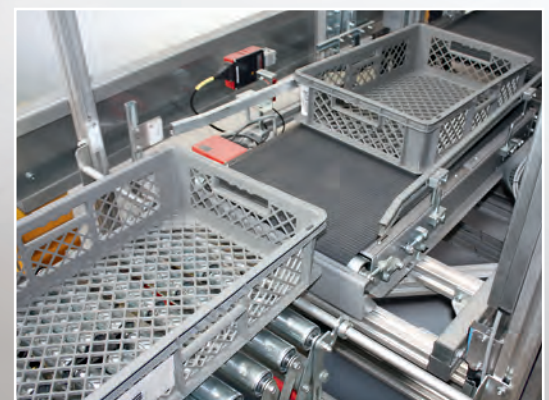
Feed station of a portal lifter with transfer onto the pivoting infeed conveyor, separating out the items.
