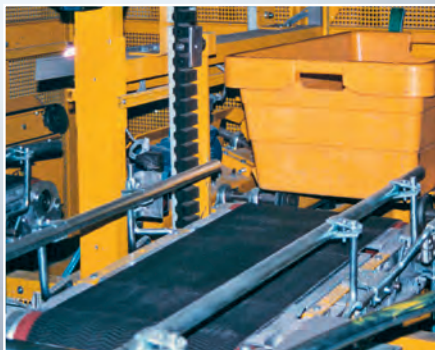
For unit loads of identical dimensions, the platforms are suspended from the rubber block chain and run in plastic guide rails for the entire circuit. This ensures smooth vibration-free running.
