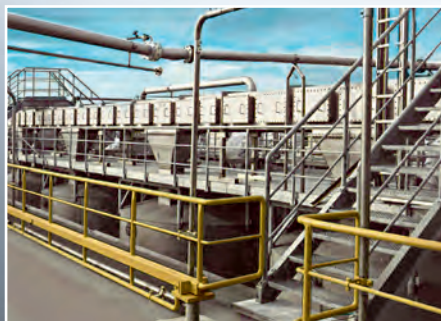
Gas-tight horizontal pendulum bucket conveyor
