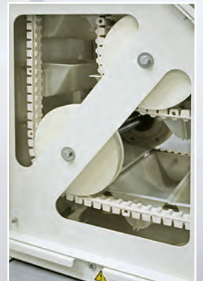
Transition from horizontal to vertical conveying
