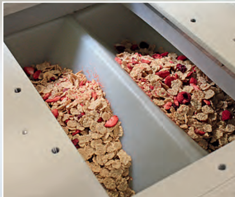
Feed point with silicon seal
