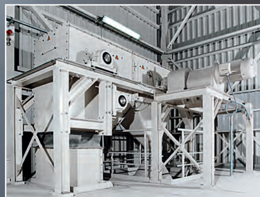
Discharge section of a WB 640 with 30 kW drive
