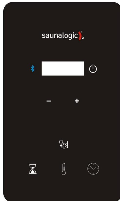
Choose the color of choice and then set lighting brightness. The brightness will be on display for 3 seconds. Press the + or - icons to increase or decrease the light setting. Setting options are 25, 50, 75, and 100% light output.
