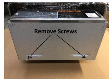
12. Lay the heater on its back and remove the two #8 screws that secure the bottom cover plate. (save screws for re-installation)
