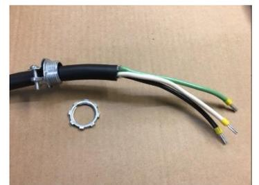
14. Insert the cable into the open hole on the back of the electrical enclosure and secure using the retaining nut from the first step. Tighten nut to prevent the strain relief from moving.
