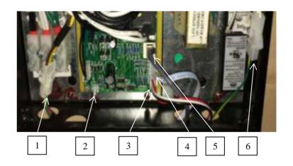
Step 4: Connect all the quick connections according to the picture and installation manual into the CB-PK Box.
