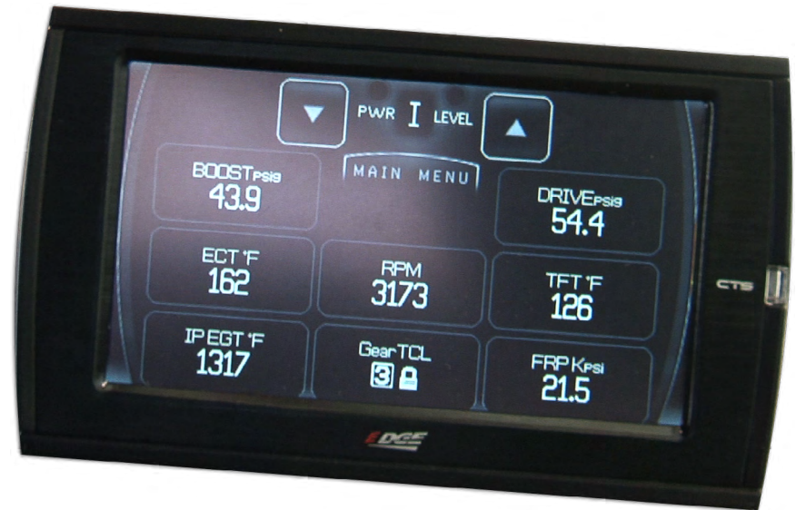
The EDGE CTS monitors horsepower, torque, boost and engine gas temperatures.
