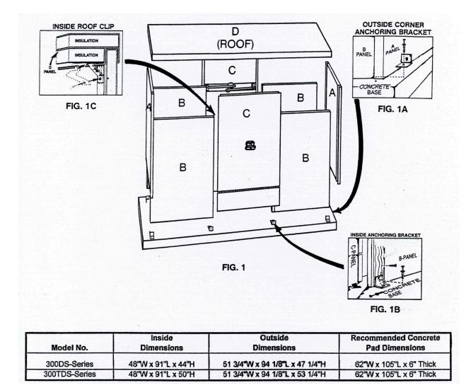
1. Center a "6" thick concrete base around installed BFP.
