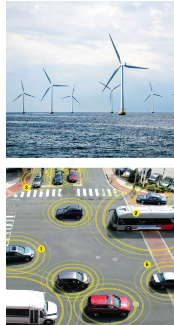
Figure 15: IIoT applications with many data items. IIoT systems often produce far too much data to send everything to every possible consumer. “Gust control” in a wind turbine farm, for instance, needs weather updates from the turbines immediately “up wind,” a specification that changes with time. Traffic control systems are very interested only in vehicles approaching an intersection. These applications require the architecture to provide selective data availability, so only the right information loads the network and the participants.
