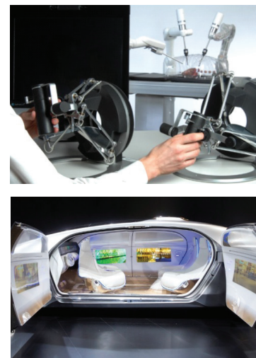
FIGURE 14: IIoT real-time applications. To provide quality feel to surgeons, distributed control loops for medical robotics must run at rates up to 3 kHz and control the “jitter” to only tens of microseconds. Similarly, autonomous cars must react fast enough to safely control the vehicle and prevent collisions. These fundamental performance needs imply a system architecture that does not send data through intermediaries.
