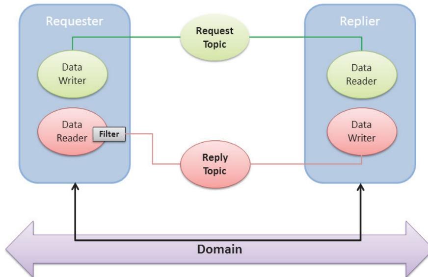
The Reply Topic filters samples so replies are received by exactly one *Requester*—the one that wrote the related request sample.
