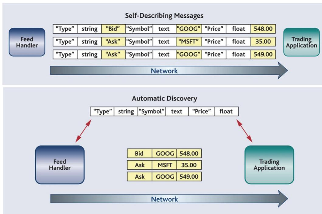
*Connex* exchanges data type definitions, such as field names and types, once at application start-up time. This increases performance and reduces bandwidth consumption compared to the conventional approach, in which each message is self-describing and thus includes a substantial amount of metadata along with the actual data.
