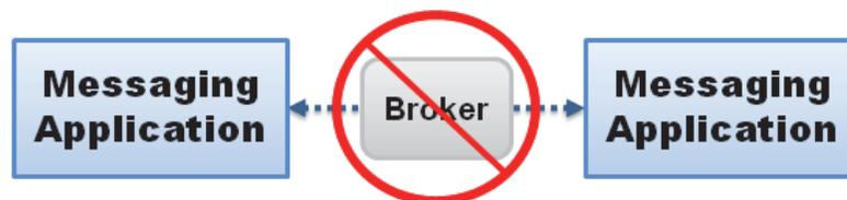
*Traditional message-oriented middleware implementations require a broker to forward every message, increasing latency and decreasing determinism and fault tolerance. RTI's unique peer-to-peer architecture eliminates bottlenecks and single points of failure.*
