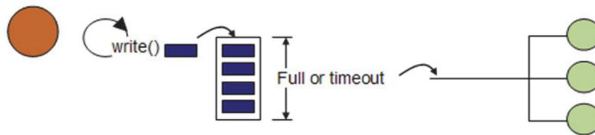
*RTI collects samples in a batch until the batch is flushed.*
