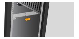
1-4 Carefully lift the SnapStream appliance and insert the ends of the inner rails into the rail assembly. Be sure to fully extend the rails before installing them. The appliance should slide in and out smoothly on the rails.
