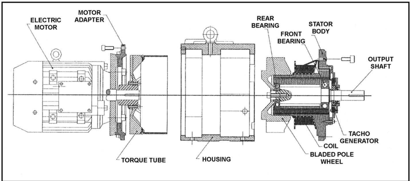
Typical Assembly Drawing of DCD Drive
