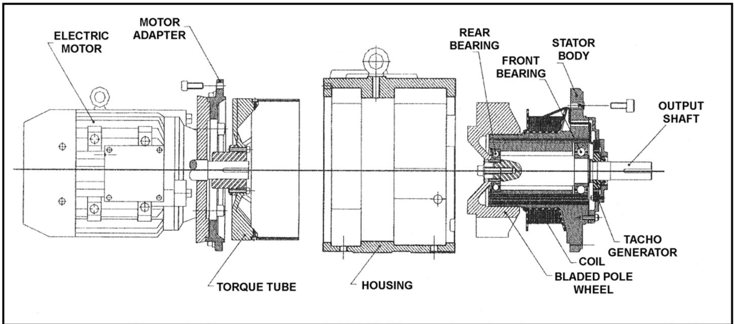
**Typical Assembly Drawing of DCD Drive**
