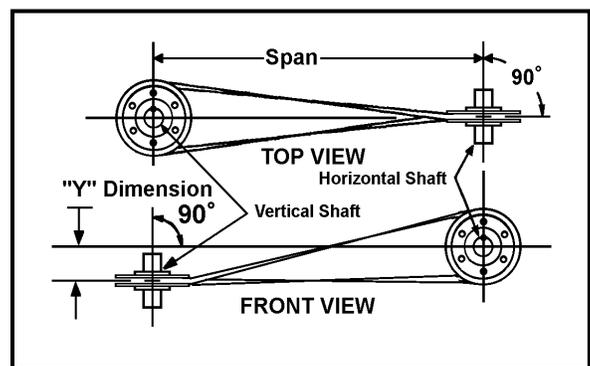
Perpendicular Shaft Alignment Figure 3-5
