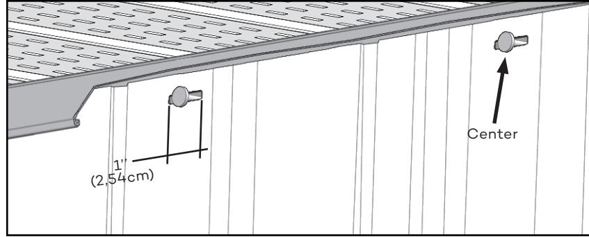
If you need to attach the section in an area other than the installation hole, create a 1"(2,54 cm) long slot to allow nailing. Always nail in the middle of the slot.
