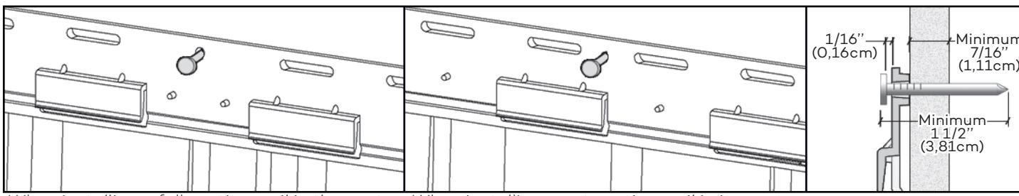
When installing a full section, nail in the center hole first.
