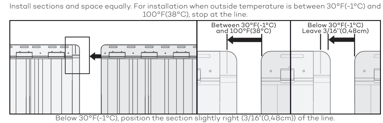
Below 30°F(-1°C), position the section slightly right (3/16"(0,48cm)) of the line.
