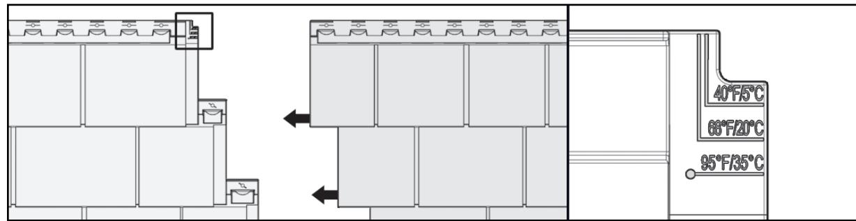
Below 40°F(5°C), position the section slightly right (1/16"(0,16cm)) of the 40°F(5°C) temperature line.
