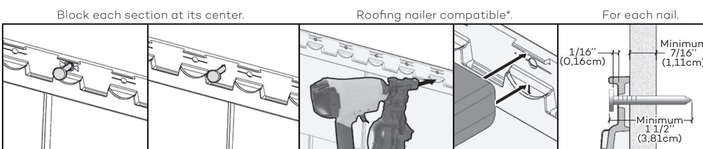
When installing a full section, nail in the center hole first.
