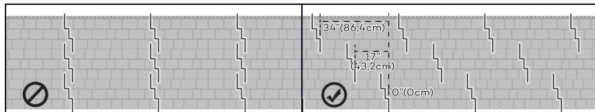
Alternate the joints between rows. For a nicer look, we suggest alternating the cutting distance of the first section of every row from 0"(0cm) - 17"(43,2cm) - 34"(86,4cm).
