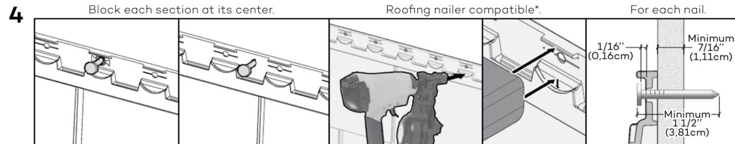
When installing a full section, nail in the center section, nail in its center hole first.      When installing a cut section, nail in its center roofing nailer, adjust its tip at the highest position and the air pressure as shown.      For each nail, leave a gap between nail head and section. When using a roofing nailer, adjust its tip at the highest position and the air pressure according to the substrate in order to leave the required gap.
