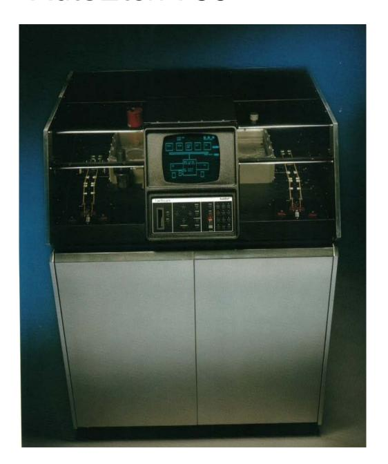
The AutoEtch 790 has been designed specifically for processes requiring good control over anisotropy including Tungsten etch back applications.
