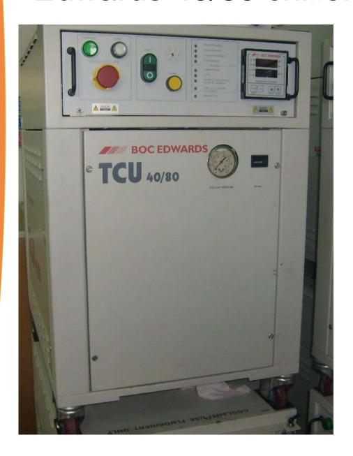
The BOC Edwards TCU 40/80 chiller is designed to meet the stringent requirements for the cooling of wafers during etch or other semiconductor processes. They are suited to all processes - typical applications include the cooling of electrostatic chucks, quartz windows, chamber domes and walls.
