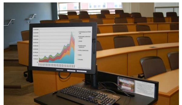
Crestron tablet provides system control and annotation at the lectern
