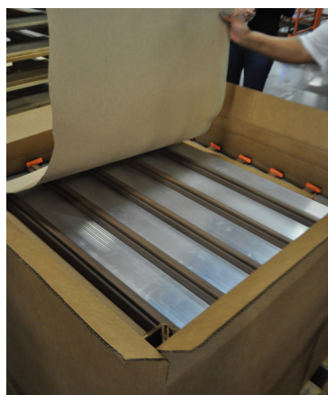
4) After the initial layer of sills has been removed from the box, remove protective packing layer to expose next layer of sills.
