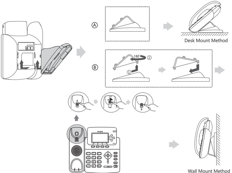
**Note:** The hookswitch tab has a lip which allows the handset to stay on-hook when the IP phone is mounted vertically.
