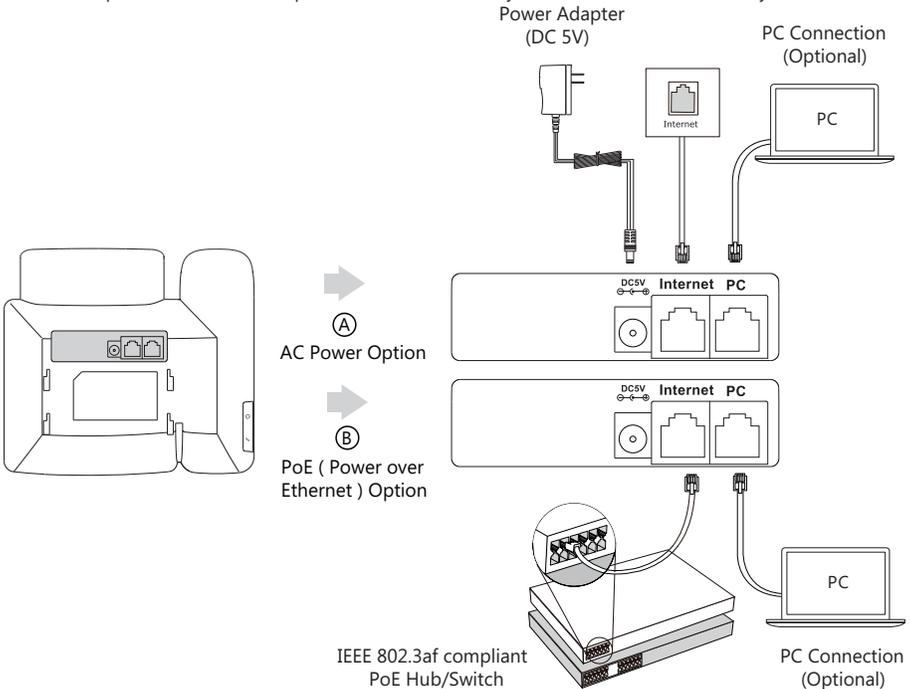
Note: The IP phone should be used with Yealink original power adapter (5V/600mA) only. The use of the third-party power adapter may cause the damage to the phone. If you are connecting a PC to your phone, we recommend that you use the Ethernet cable provided by Yealink.
