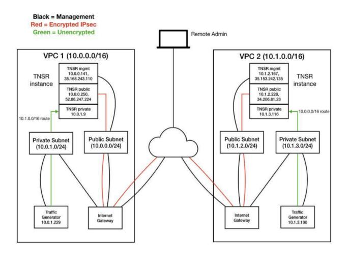
Tests are performed on the AWS Marketplace with private EC2 instances. Each IPsec endpoint and traffic generator host runs on a C5.xlarge instance running CentOS 7.4. Each instance is equipped with four CPUs and 8 GB of RAM and Elastic Network Adapters (ENA).
