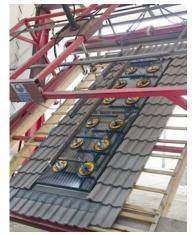
Wind uplift pressures are higher when solar is roof integrated and the wind resistance of some integration products is not high enough even for low-rise scenarios (see chart).
