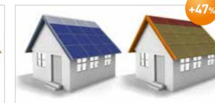
**Standard sized modules** can cover the roof in its width, but not in its height. **The slim N245 module** perfectly fits in the remaining tight space.
