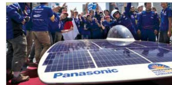
**Solar car:** The "Tokai challenger" is Tokai University's record breaking solar car powered by Panasonic lithium-ion batteries and HIT® solar modules. Both technologies are optimal for solar car races because of their resilience to high temperatures and their high power output per unit area. We proudly helped the "Tokai challenger" win the 2009 and 2011 World Solar Challenge in Australia, along with the Sasoi Solar Challenge, South Africa 2012 and the Carrera Solar Atacama, Chile in 2014.
