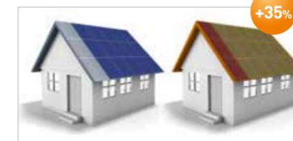
**Standard sized modules** can't entirely cover the roof in its width. **The slim N245 module** perfectly fits in the remaining tight space.
