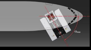
Models with an oversteering protection system measure the forces and avoid damage to the nose gear.
