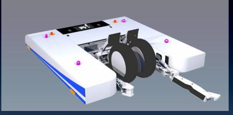
2. The hydraulical door closes. If necessary the sliding table is adjustable for fitting smaller nose wheels.
