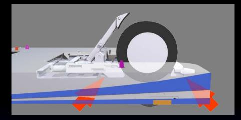
3. The sliding table presses the nose wheel towards the closed hydraulical door until a specified pressure is reached.
