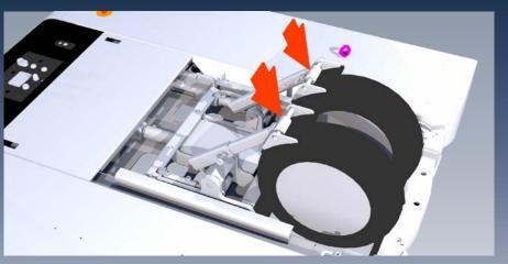
5. The Securing Paddels lowers down and clamps the nose wheel gently and safely - ready for moving the aircraft.
