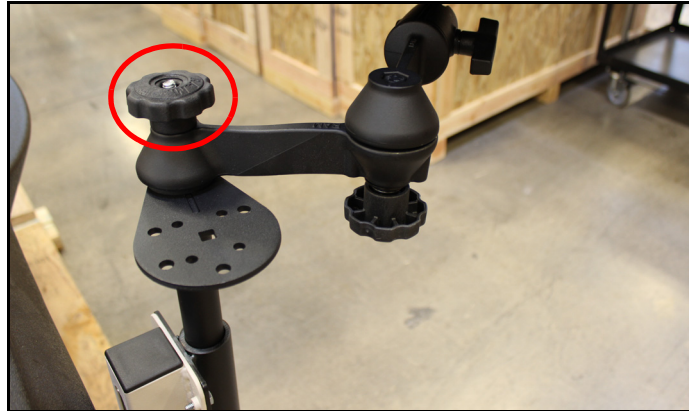
Figure 16 Attaching Swivel Arm to Mount Arm
