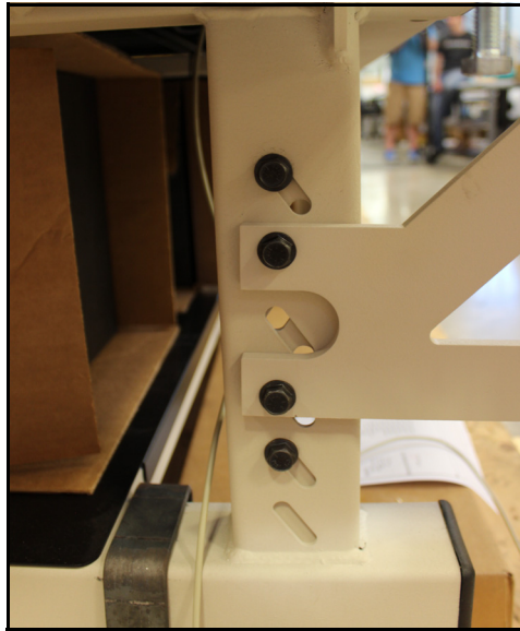
Figure 14 Attaching Laptop Arm Frame to CubiScan Frame
