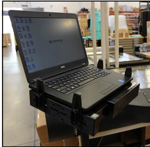
Figure 13 CubiScan 150-T with Laptop Tray Arm Attached
