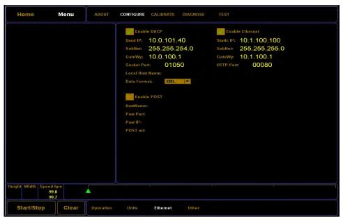
Figure 22 Configure Ethernet menu
