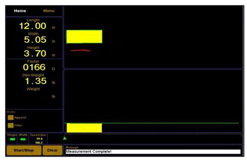
Figure 16 Box measurement results
