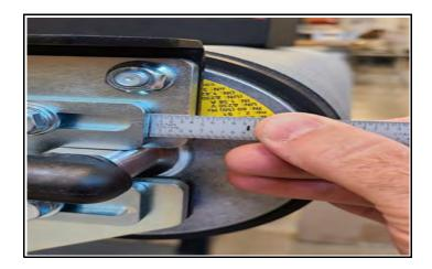
Figure 32 Tension measurement
