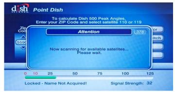
NOTE: If you see an X in the place of the satellite information (110, 119, 129) at this step, reposition your satellite antenna and then select 'Test.'
