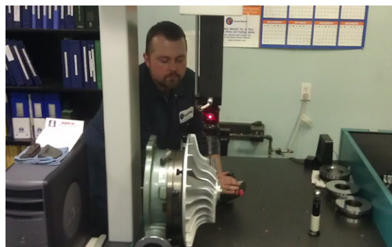
Corey Halloran, Chipco's QA/CMM specialist, takes points on an impeller to create a new program in MAX-PAC.
