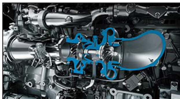
An Exhaust-Gas Turbocharger for HD Daimler CV Engines. (Image Courtesy of ATZelektronik)
