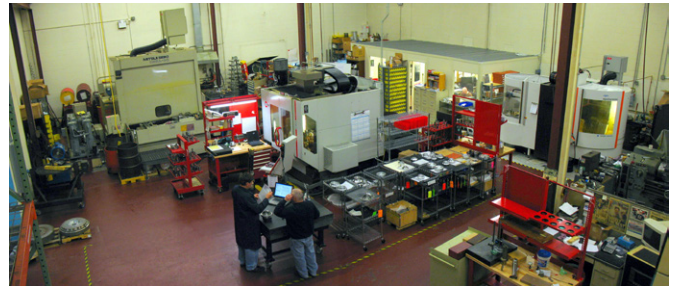
Concepts NREC workshop with Hermle C40 U five-axis machining center used for rough and finish-machining vane rings for the aero fixed stator case.
