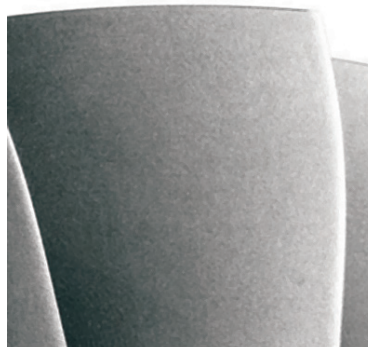
The toolpath accuracy of MAX-AB greatly improved surface finish and eliminated most post-machining finishing.
