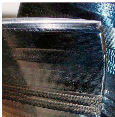
Toolpaths generated with general CAM software resulted in rough surfaces that required hand finishing.
