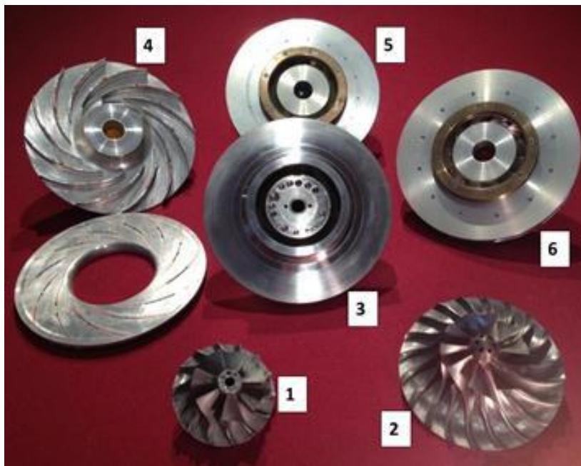
Figure 7. Consortium Impellers: [1] – High N_s ; [2] – Medium N_s ; [3] – Low N_s . The remaining (Nos. 4 – 6) are low N_s pump impellers comparable to item [3]
