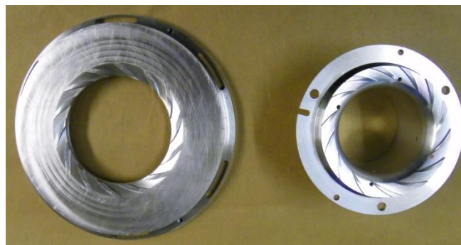
Figure ES6. The grooved cover – impeller cover is on the right, which mates with the 25% pinch diffuser front cover shown on the left
